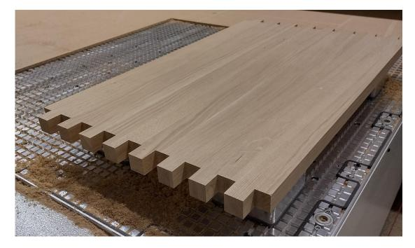
• Corner dove tail joint of solid wood (here aplied on table level 5/5)
